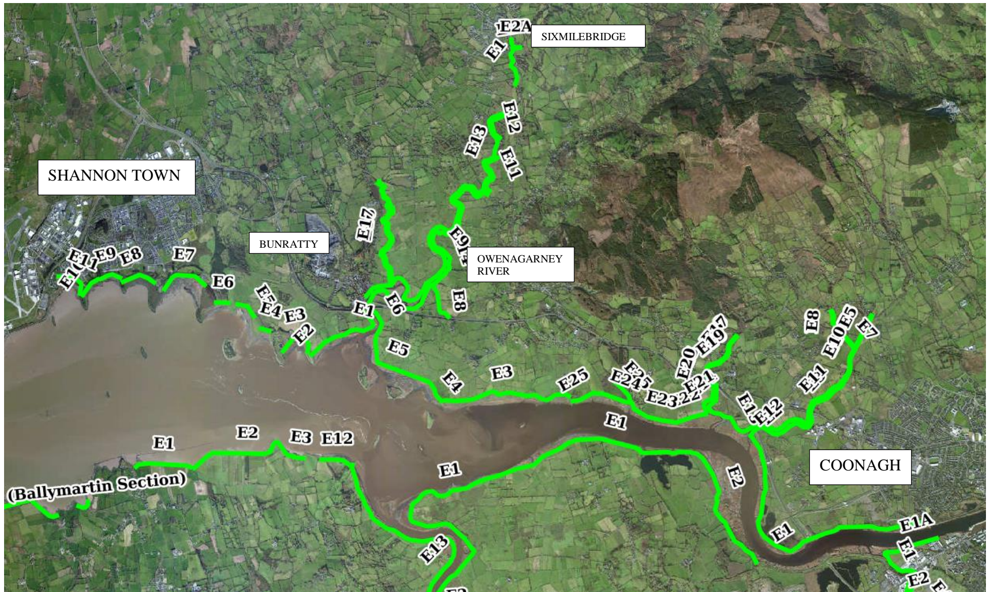
Figure 1: Map of Study Location showing OPW Embankments to be assessed (north of Shannon Estuary only)
