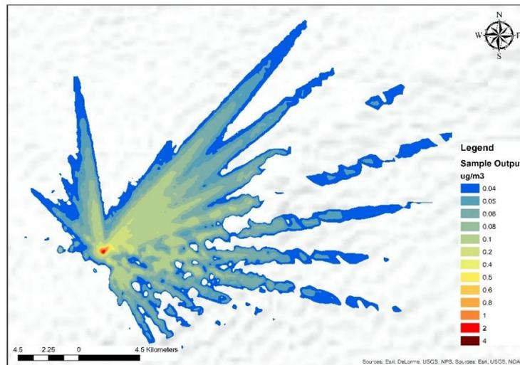
**Figure 1: AERMOD model scenario for ammonia from a broiler farm presented in ArcGIS using EPA emission factor (EPA, 2016) and average ventilation rate from SCAIL (Hill et al. 2014).**
