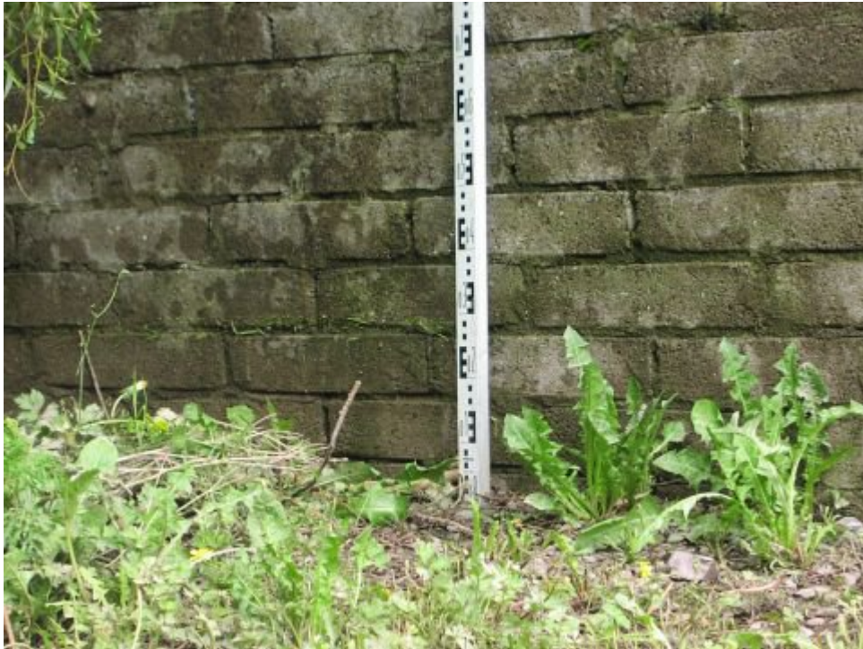
Photo showing tide line at about 0.27m on staff on inside of wall at exit from hotel grounds near north end of flood extent
