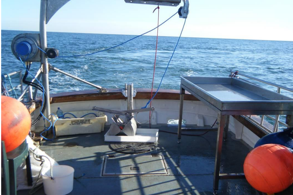
Plate 20: Van-Veen grab ready for deployment over the Bray Bank in May 2010.
