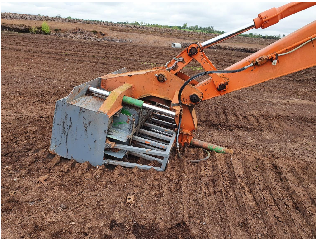
Photo 2: Attachment for excavating sod peat noted.
