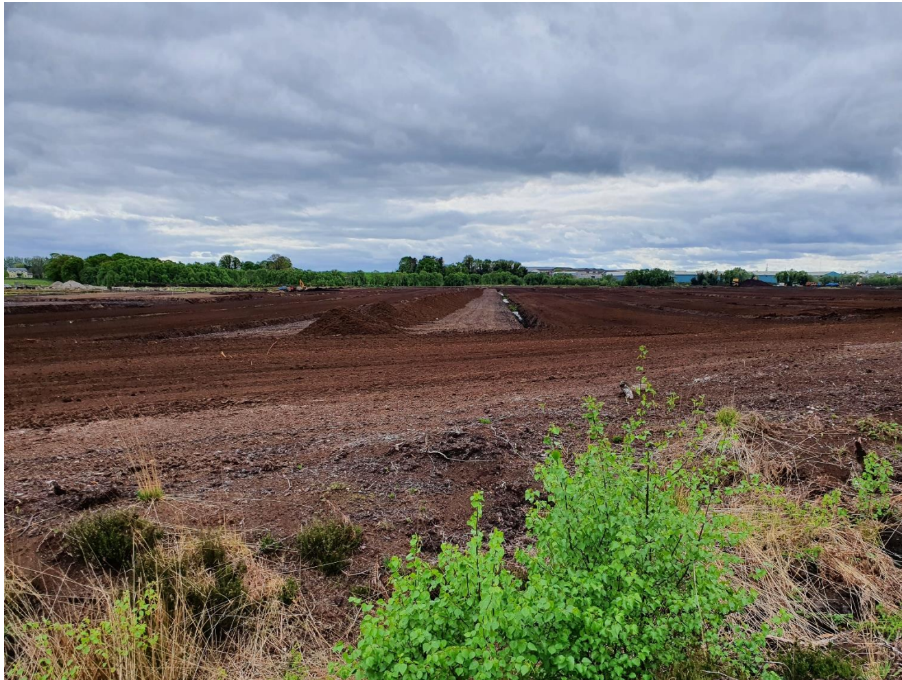
Photo 1: Stockpiles of milled peat awaiting collection and haulage to the loading area.
