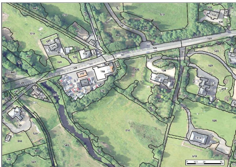
Figure 5.3: Examples of Artificial Surfaces classes in a non-urban setting, including Buildings (110), Ways (120) and Other Artificial Surfaces (130).
