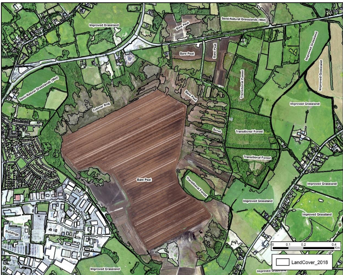
Figure 5.17: Example of the NLC 2018 map showing areas of Cutover (630) and Bare Peat (640).
