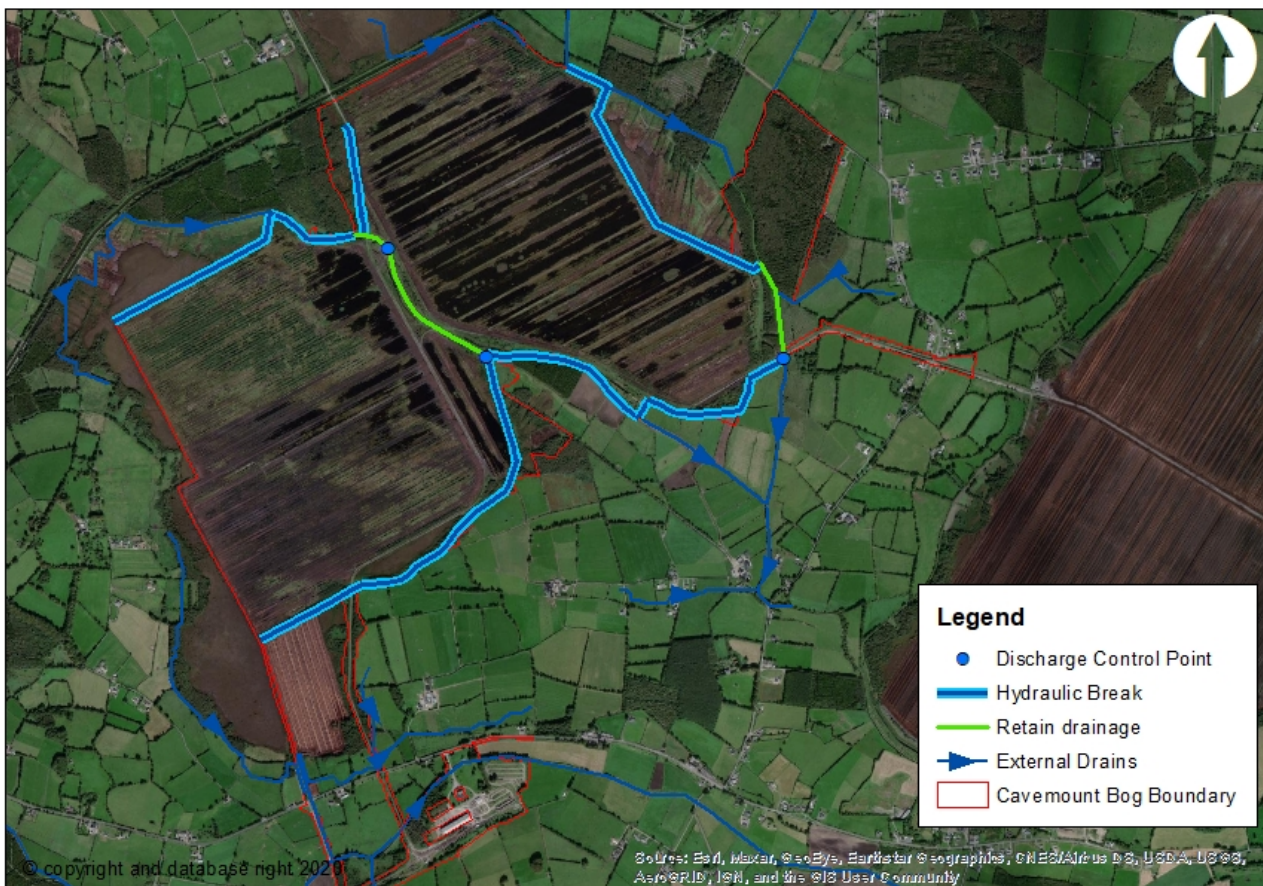
Figure 5.1 Key drainage features for Cavemount Bog
