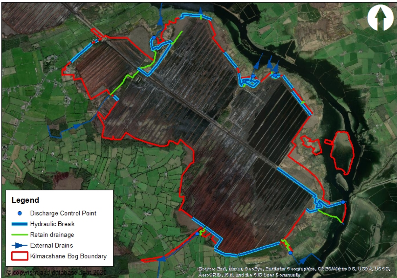
Figure 5.1 Key drainage features for Kilmacshane Bog
