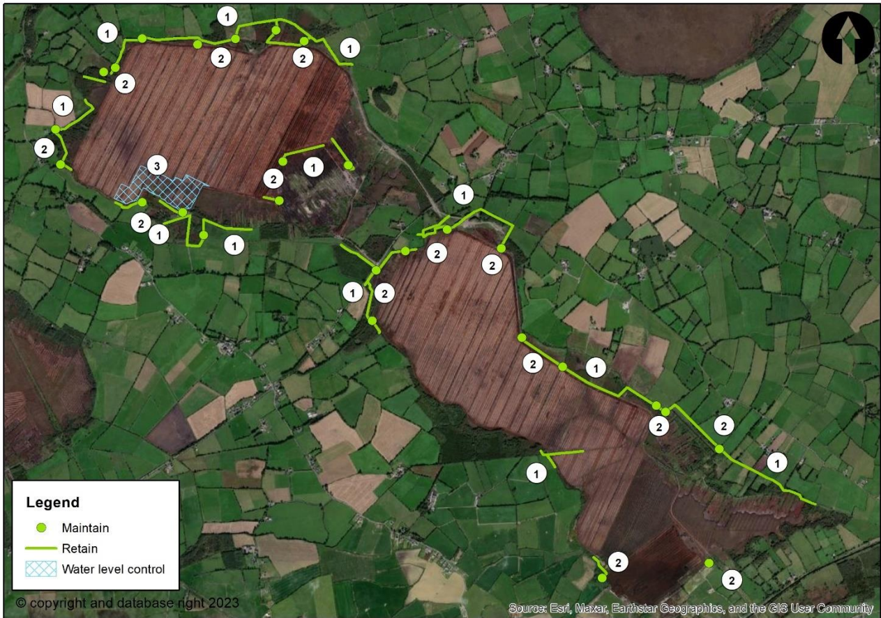
Figure E- 4: DMP measures for Daingean Rathdrum and Daingean Derries Bogs (1-Retain drains, 2-Maintain outlets, 3- Water level control)
