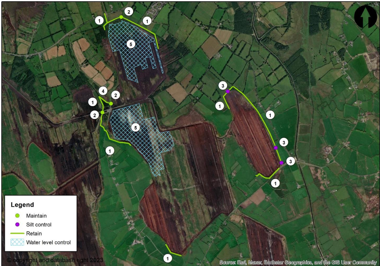
Figure E- 4: DMP measures for Derryadd East Bog (1-Retain drains, 2-Maintain outlets, 3-Silt control, 4-retain drain outside bog boundary, 5- Water level control)
