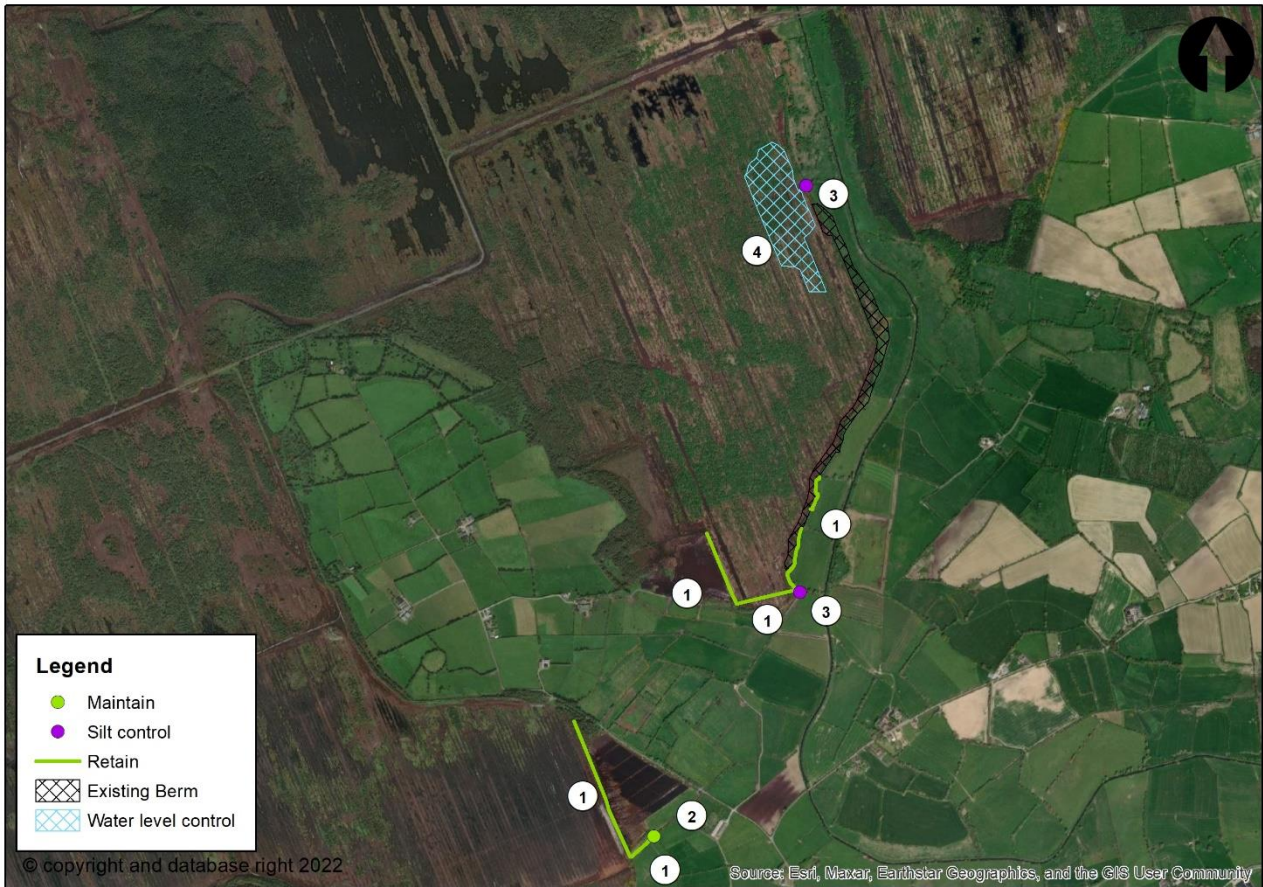
Figure E- 4: DMP measures for Drinagh Bog (1-Retain drains, 2-Maintain outlets, 3-Silt Control, 4- Water level control)
