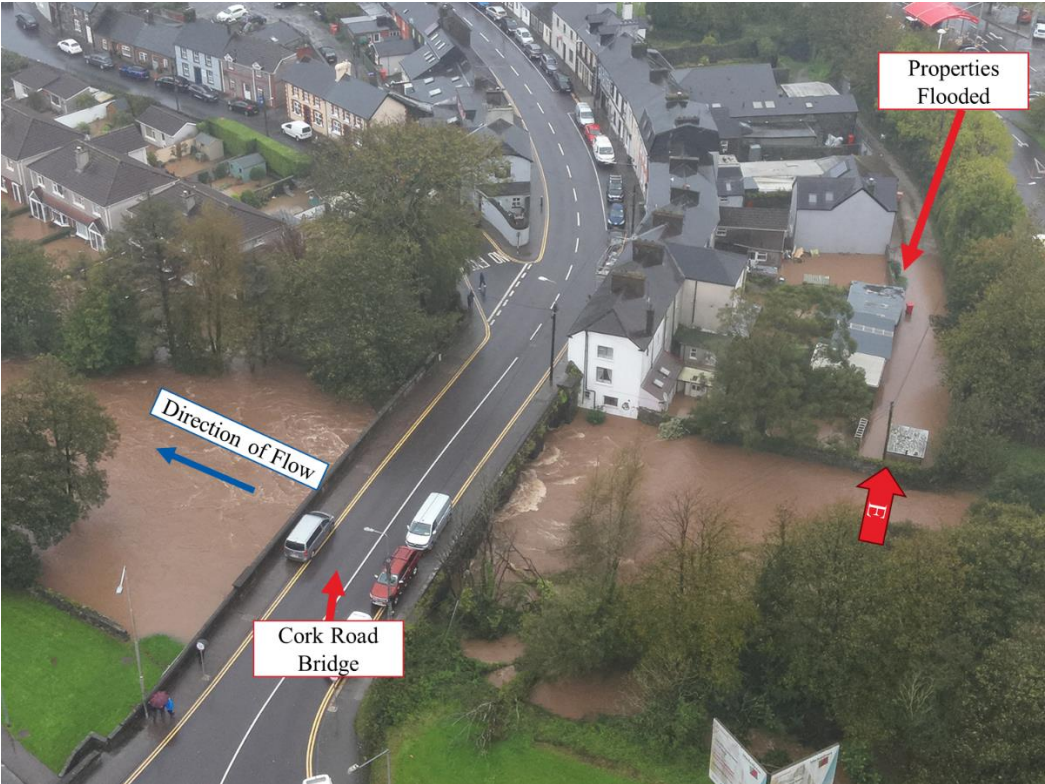
Figure 45: Flooding on Right Bank Upstream of Cork Road Bridge
