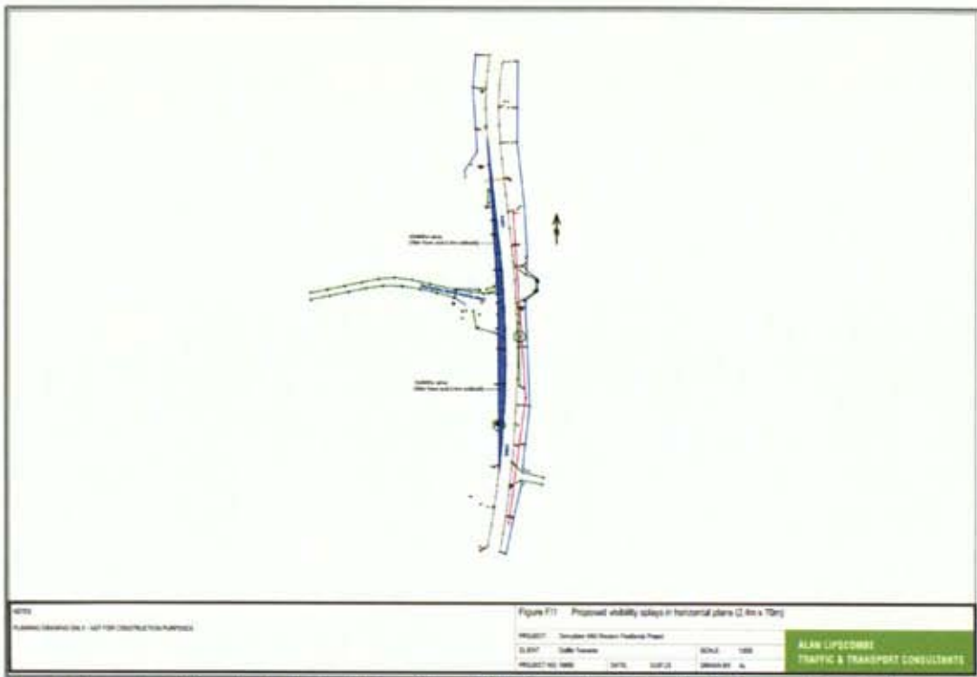
Figure 1: Proposed visibility splays in horizontal plane (2.4m x 70m) (Source Alan Lipscombe FI Response Figure F11)
