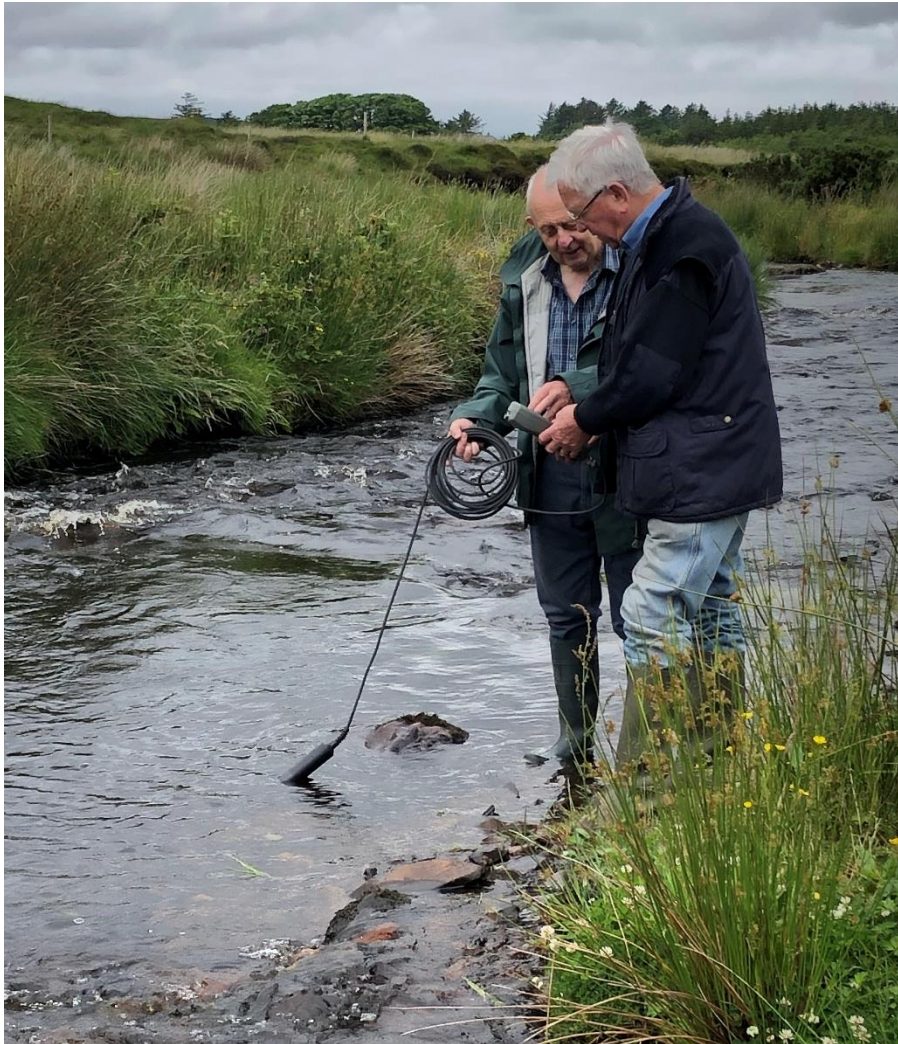
Figure 3 CAA training in use of multiparameter meter
