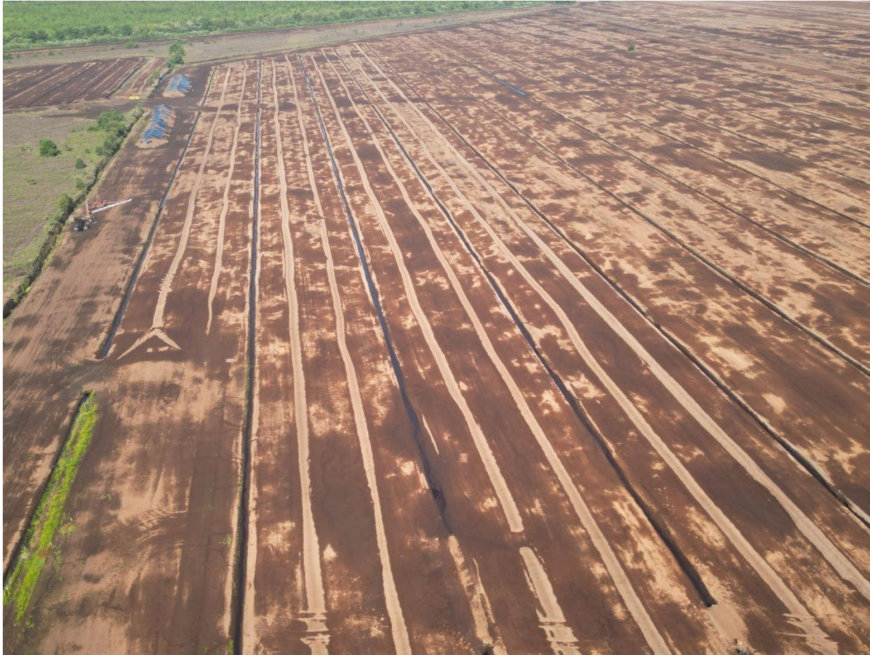
Photo 4: Ridging of milled peat noted in some of the rows at the southern end of the peatland, covered milled peat stockpiles and peat harvesting machinery noted here also.
