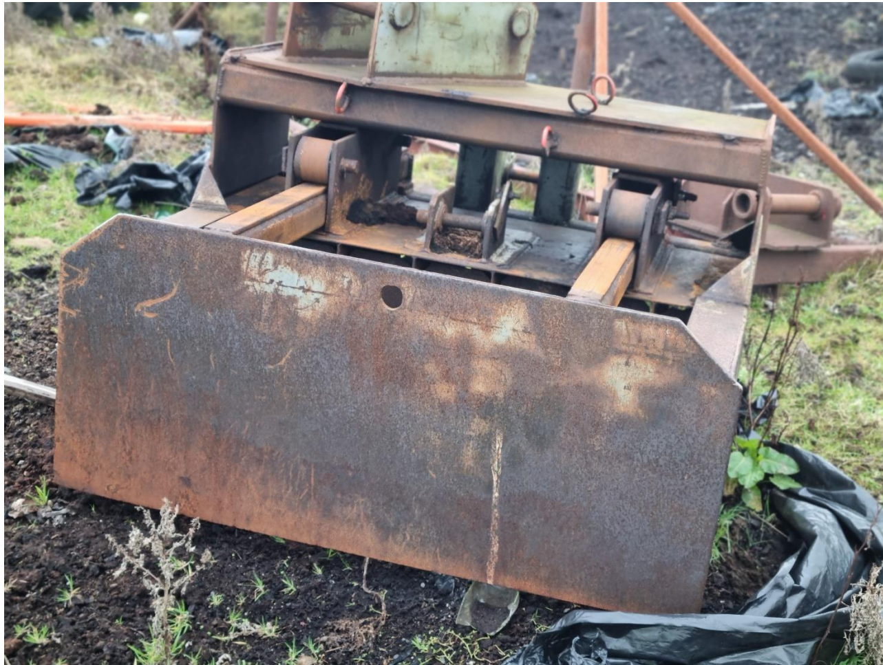
Photo 6: Photograph showing attachment for large sod peat extraction which was noted at the loading area.
