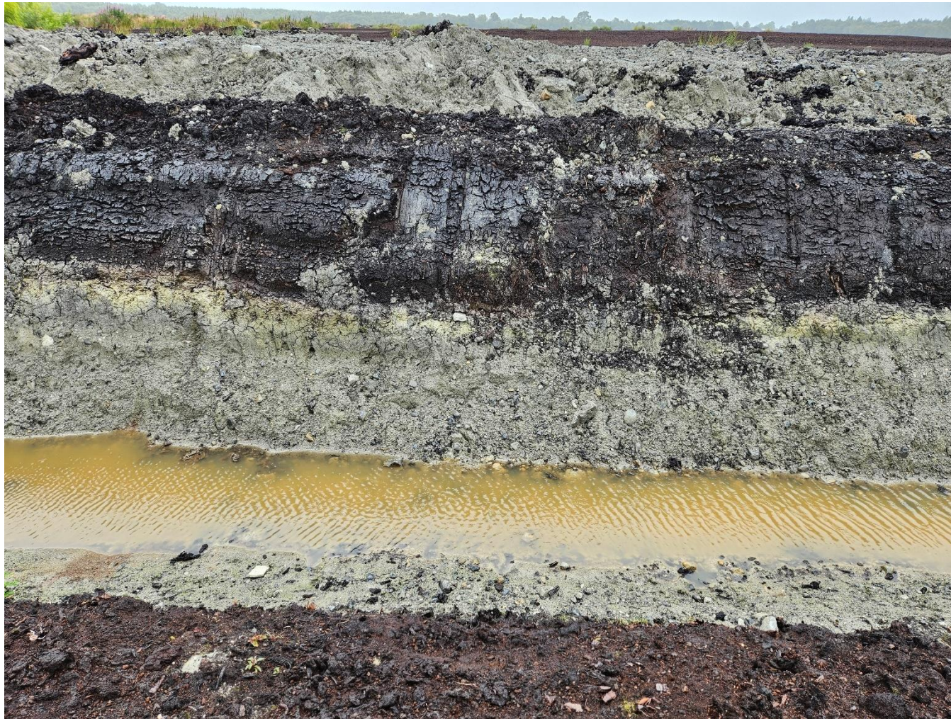
Photo 1: Photo showing the marl like materials underlying the remaining peaty deposits on the peatland.
