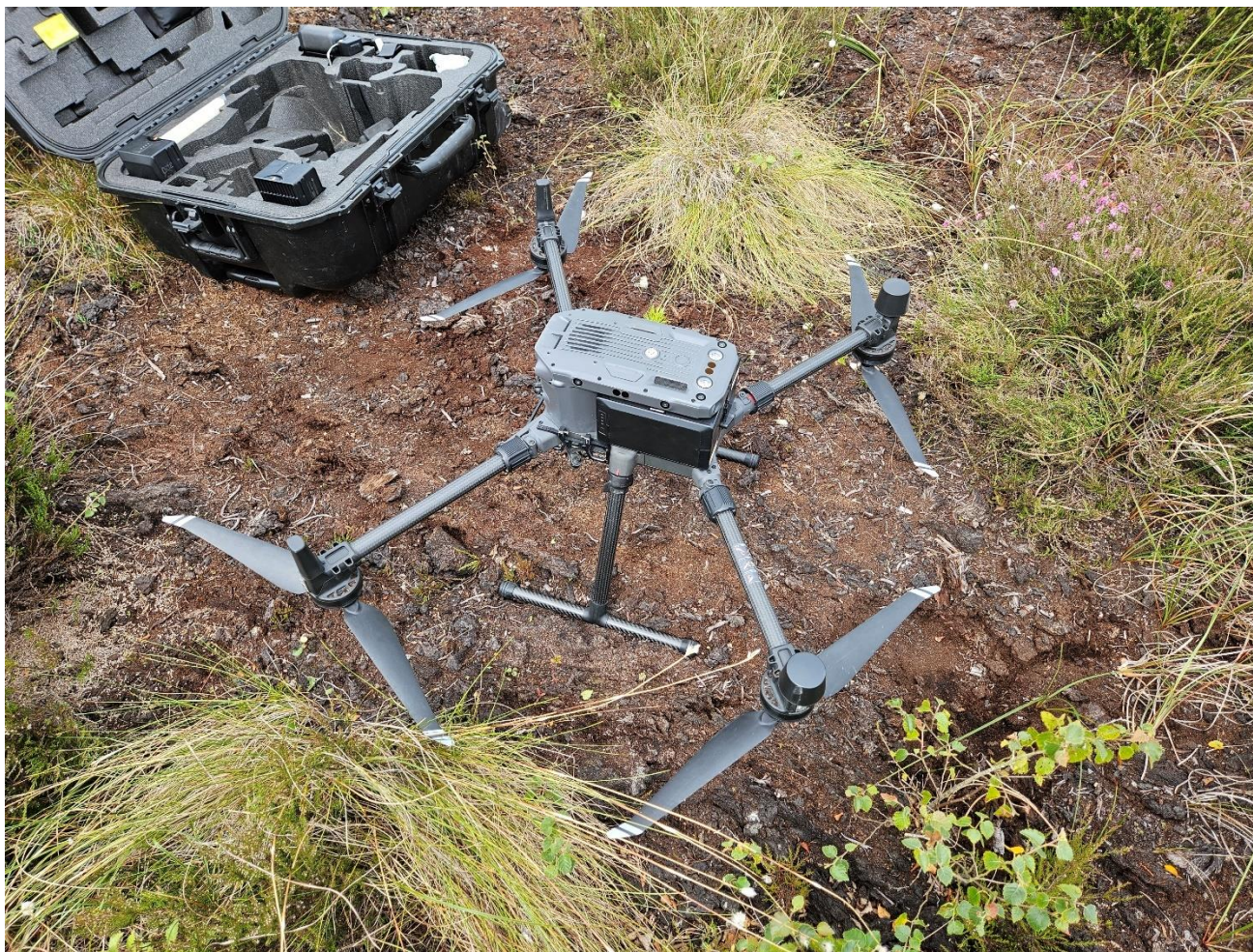
Photo 4: Photo of UAV (drone) used to carry out survey of the peatland.
