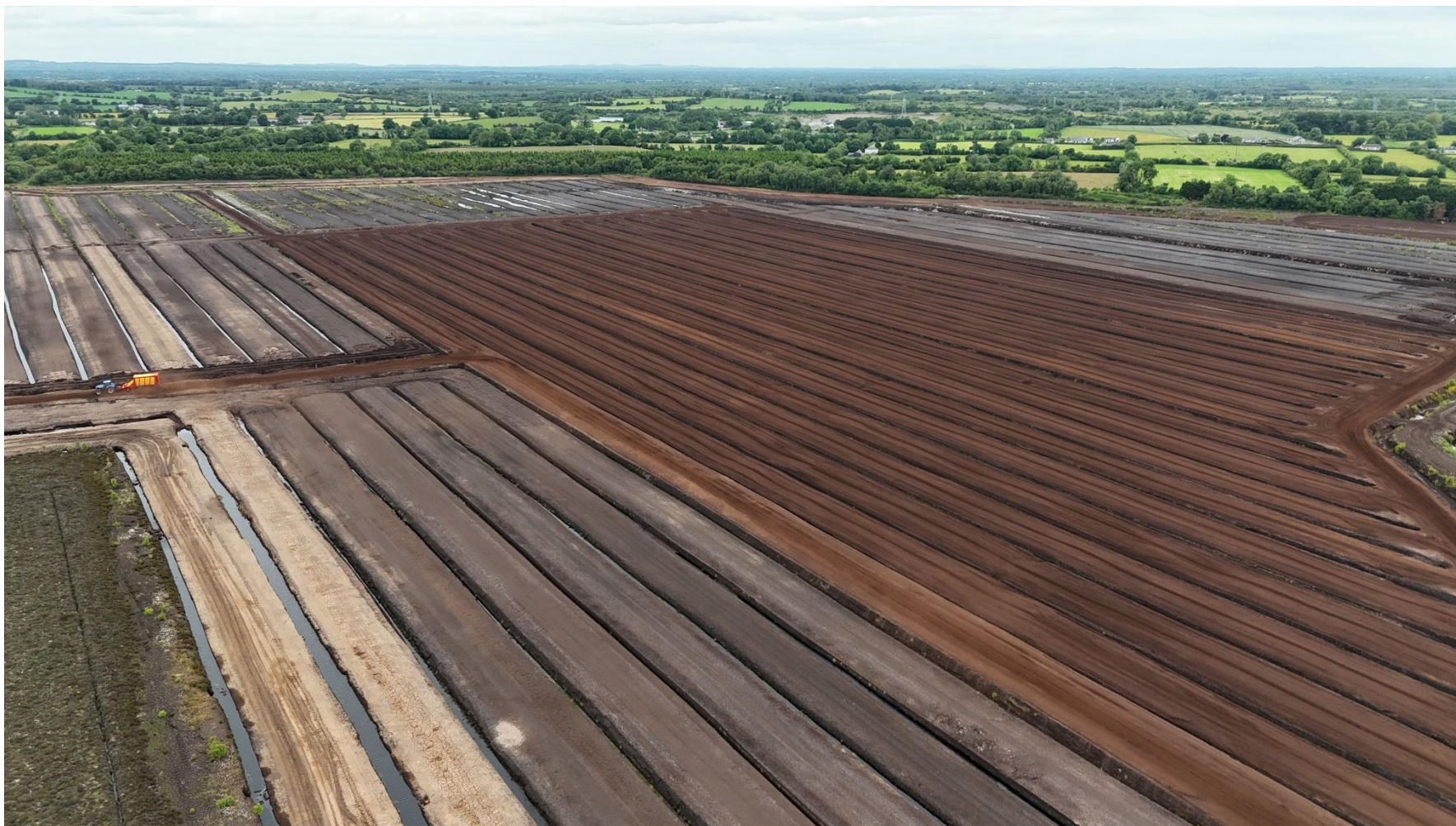
Photo 2: Photo of central part of the peatland where peat extraction had taken place recently (note dark brown colour). Also, note tractor and trailer ('Bog Hog' ) going to the South western part of the peatland to collect milled peat.
