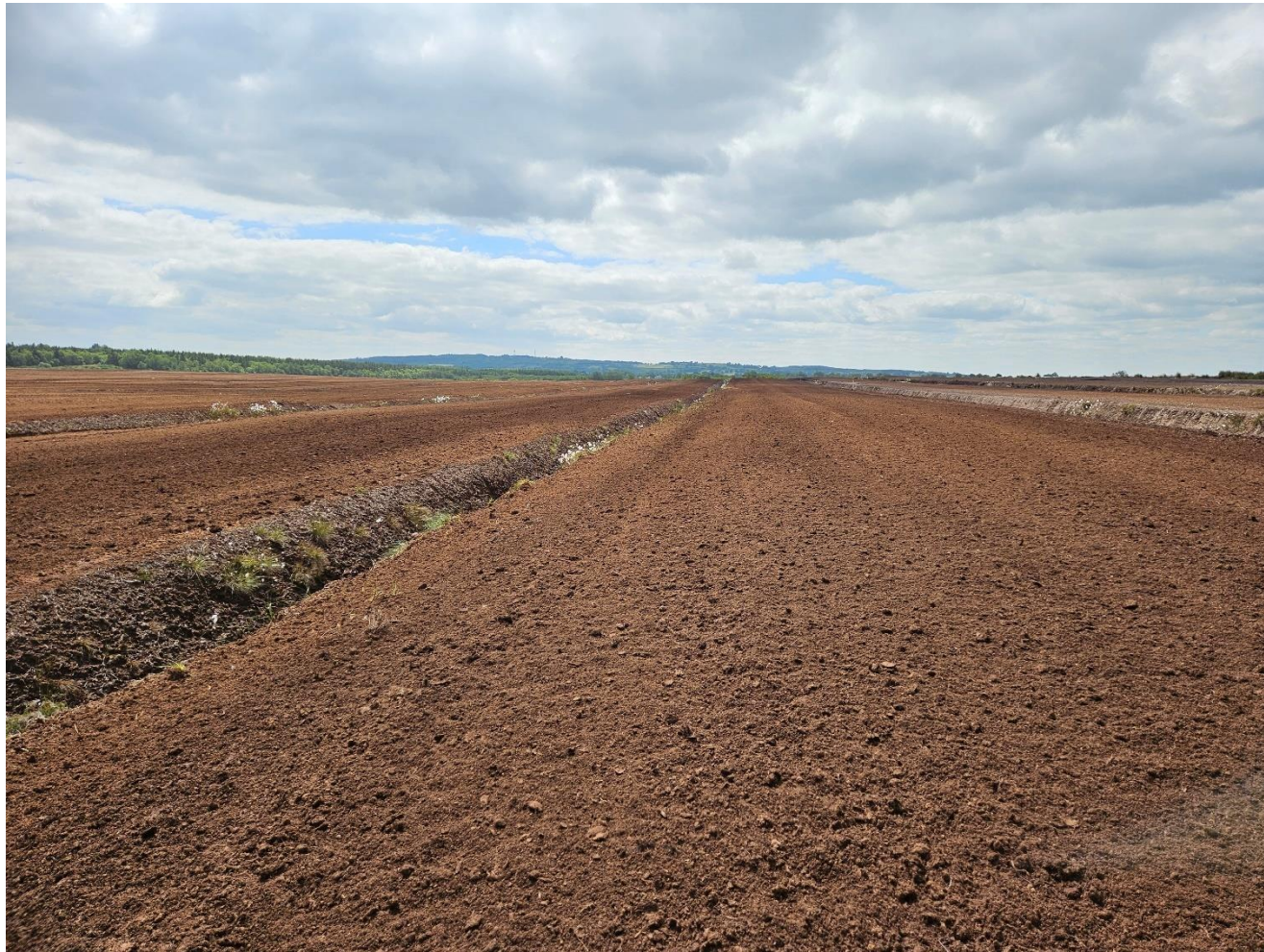
Photo 4: Recently ‘milled’ peat noted on the peatland awaiting further processing prior to collection and removal off the peatland.
