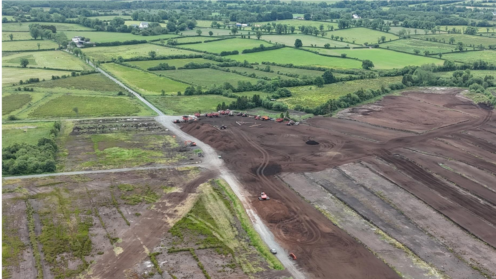
Photo 6: Stockpiles of milled peat and peat extraction and harvesting machinery noted at the loading area.
