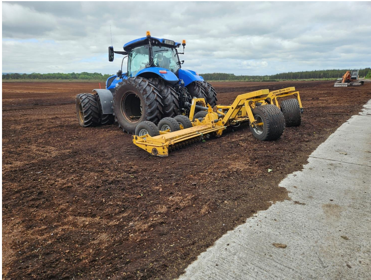
Photo 8: Photo showing milled peat extraction and harvesting equipment on the peatland.
