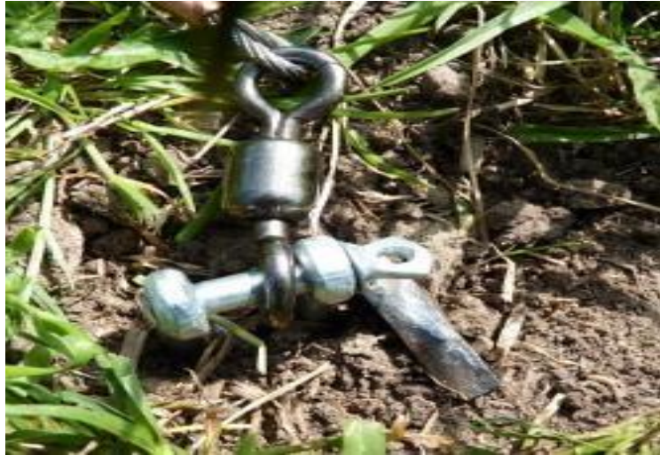
Photo 2: This model has an anchor system, which may be advantageous in open ground where there are no fixed points to secure a snare.
