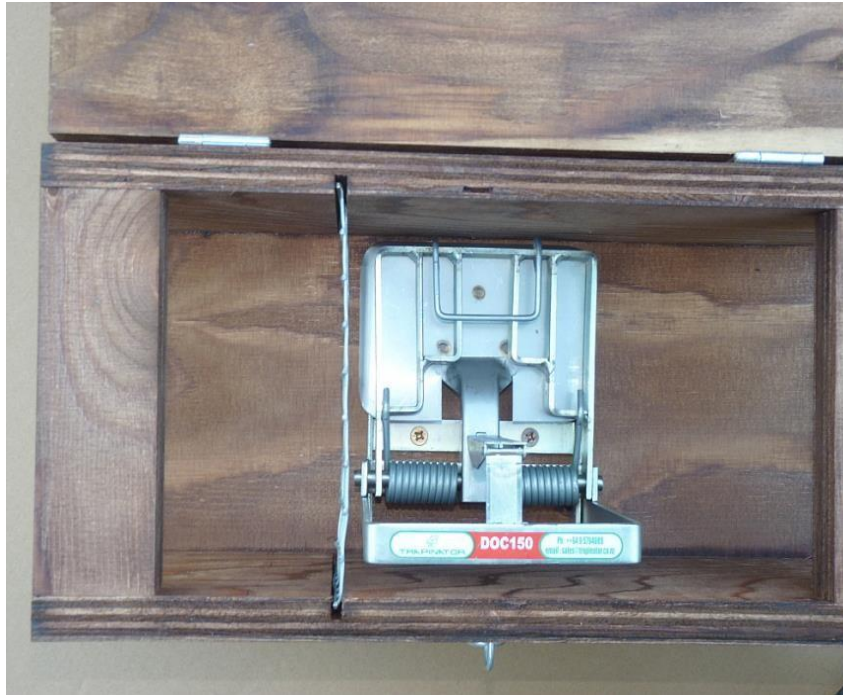
Photo 5: New Zealand Department of Conservation (Doc) approved spring trap
