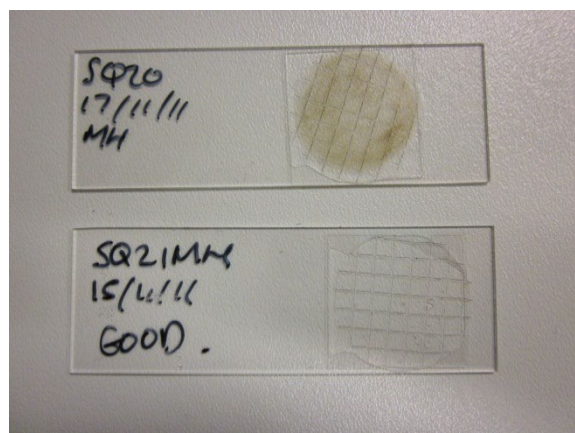
Picture 2 - An occluded filter (top) prepared from a clay soil sample. A non occluded filter is shown on the bottom for comparison.
