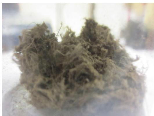
Picture 3 - The chrysotile problem of clumping – the addition of surfactants is not helpful, as the clumping is caused by the morphology of the fibres
