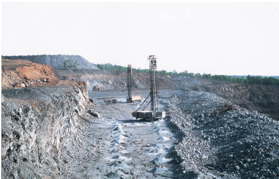
FIG. 1. The grunerite asbestos occurred along the wall and on top of the lower bench on the left.
