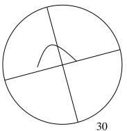
Measure curved fibres by assessing the lengths of the straighter parts of the fibre
