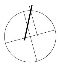
After measuring the first fibre, the stage should be rotated again to measure the second fibre.
