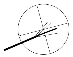
Measure the length of split fibres as the length of the longest part, and the width as the narrowest part of the fibre where all the branches are still attached to the main fibre, even is this point is outside of the graticule area.
