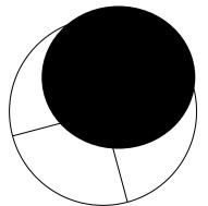
If more than half of the field is obscured by particles then the field should not be counted
