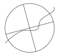
Curved fibres passing right through the graticule should be recorded as  $100\mu m$  long.
