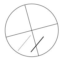
Both the fibres in this field are less than 0.5  $\mu m$  in width, and they should both be recorded as 0.5  $\mu m$ , despite one fibre being obviously much finer than the other.
