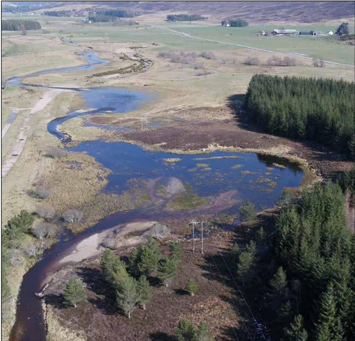
Plate 7. Example of an engineered flood plain on the, as part of river restoration measures to enhance Atlantic salmon and trout populations on the Nairn River Scotland (Image: 2017, Scottish EPA).
